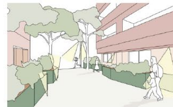
▲ 3.3.c Consider location of access, lighting and passive surveillance to communal open space.
