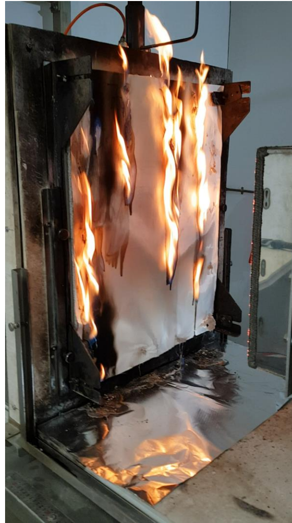
Modified AS1530.3 test on polyolefin VP PBM
